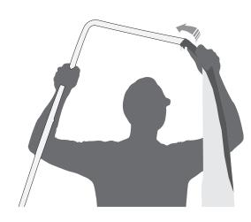
To mount the flag banner, you must first slide the printed fabric (supplied separately) through this tube system and then tighten it at the bottom by tying it to the clip.
